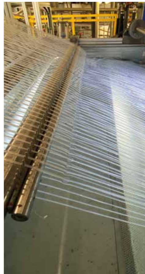
LEFT. The extrusion process is used to produce synthetic fibers at the Mapei manufacturing facility in San Cesario Sul Panaro in the Province of Modena (Italy). RIGHT and BELOW. An example of concrete industrial flooring strengthened with synthetic fibers for the Docks logistic centre in Serravalle Scrivia (Italy).
