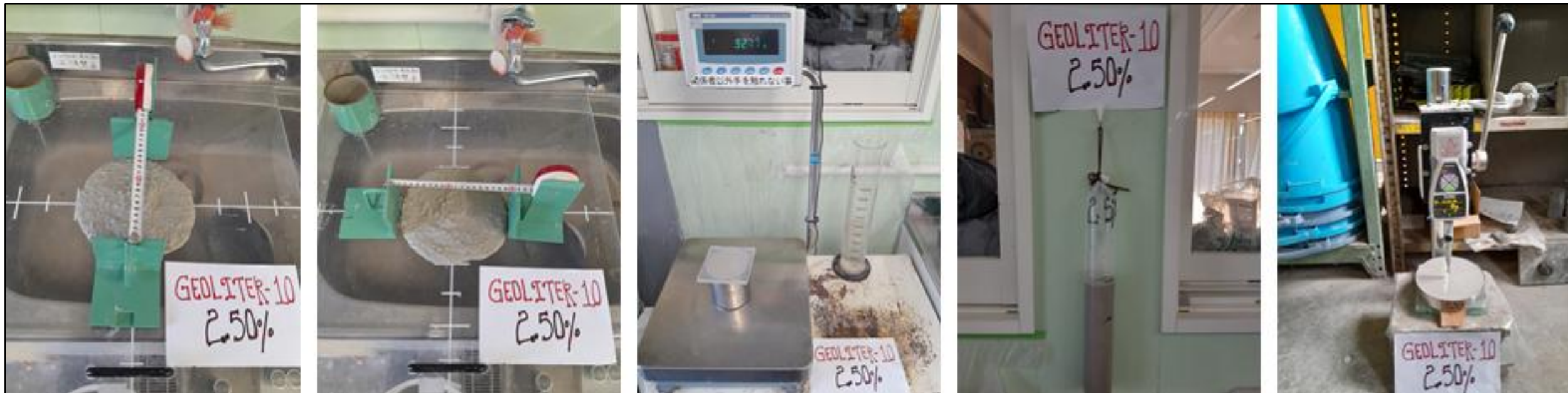
Fig. 10 Flowability, wet density, bleeding, air content, penetration, tests in Stage-IV
