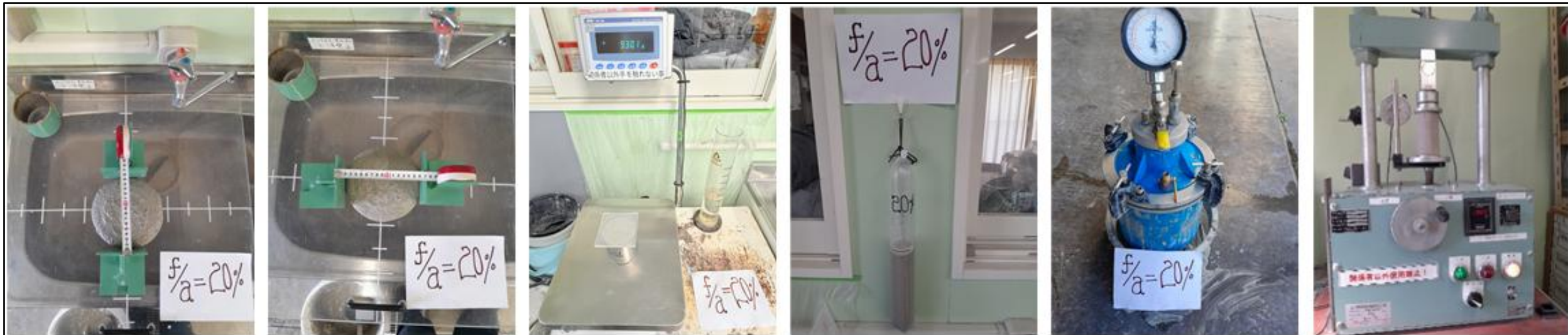
Fig. 5 Flowability, wet density, bleeding, air content, and UCS tests in Stage-II
