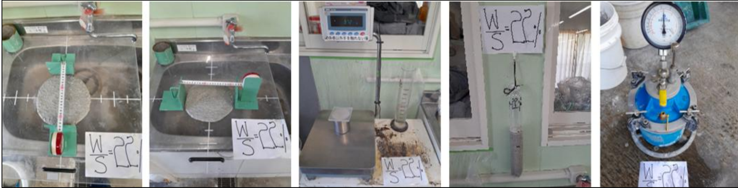
Fig. 4 Flowability, wet density, bleeding, and air content tests in Stage-I
