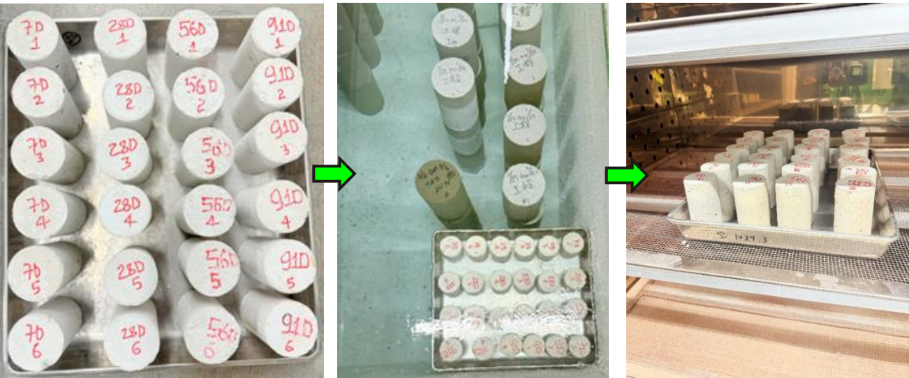
Fig. 16 Wetting-drying cycles [Specimens-wetting in water tank-drying in oven]
